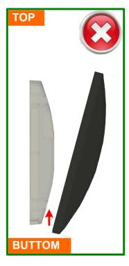
Above picture shows the correct direction (TOP) that outer housing needs to be applied.
